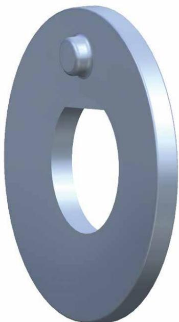
The special FKL spring washer prevents the shaft turning at the nut tightening and due to its spring properties provides 6 tons of axial clamping force.
